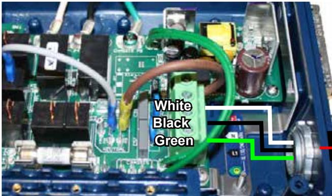
To convert, remove the cord from the terminal block and replace with White, Black and Green #10 wires and connect to 30 A GFCI Subpanel.
