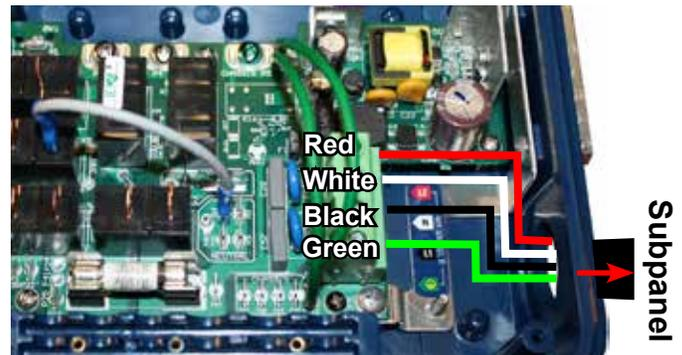
To convert, remove the cord and brown jumper wire from the terminal block. Remove other end of brown wire from connector and remove from box. Place Red, White, Black and Green #8 wires onto terminal block and connect other end to 40 A GFCI Subpanel.
